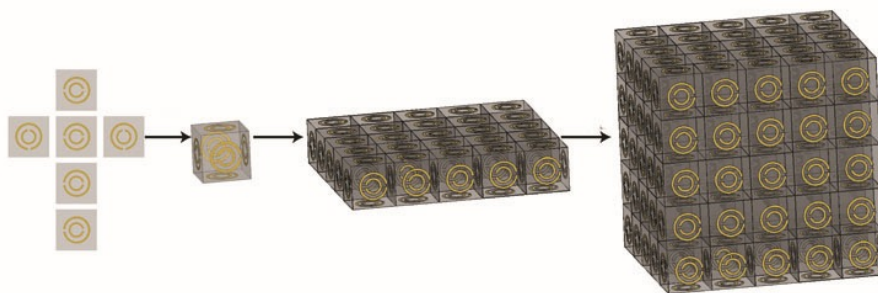
Figure 8 Conceptual schematic of the self-assembly of metamaterials with precisely patterned nanopolyhedra. Image credits: Jatinder Randhawa (Gracias Laboratory, JHU).
